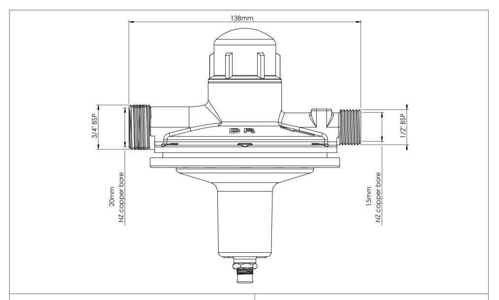
Pressure reducing valve (feed valve) FV
